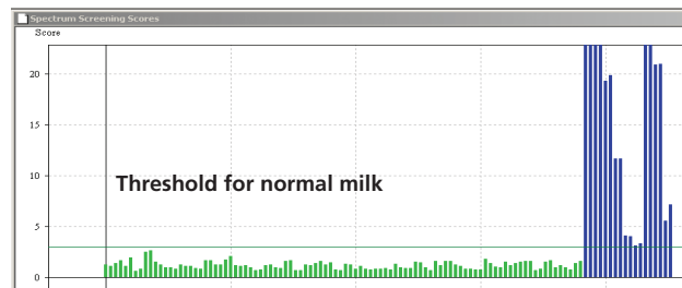
Detail of display showing preset warning level for urea content in milk samples. Samples exceeding the threshold are shown in blue.
